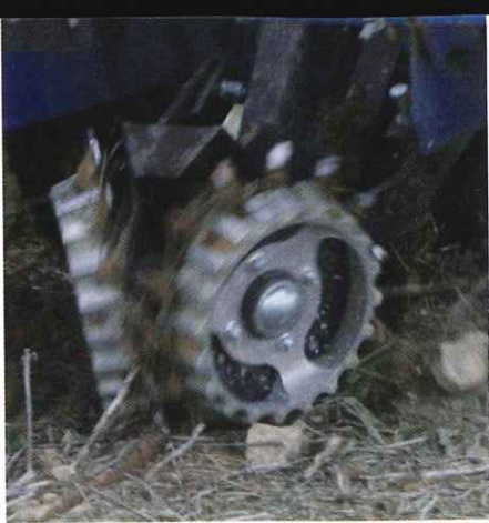
MOVE OBSTACLES. Residue managers push clods of dirt to the side so planter units do not bounce and drop seed at a poor depth.
