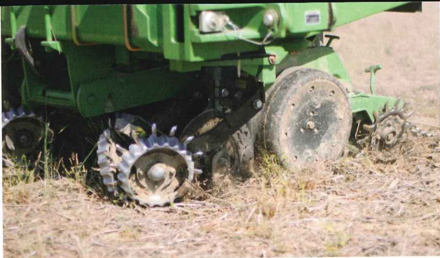
LESS DIGGING. Floating residue managers equipped with side treader wheels improve the flotation of row cleaners and prevent digging of loose, dry soils.
