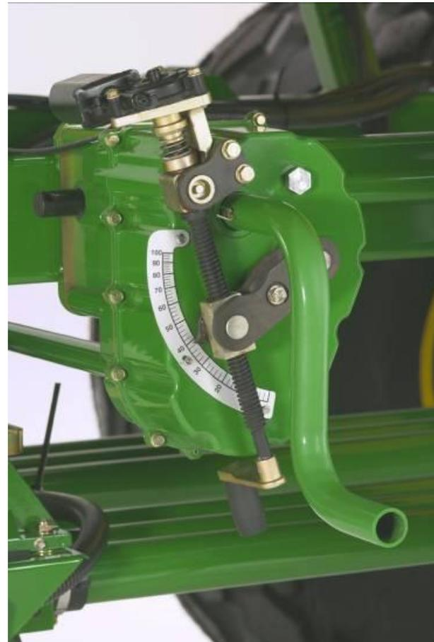
**Variable rate motor w/ transmission**
