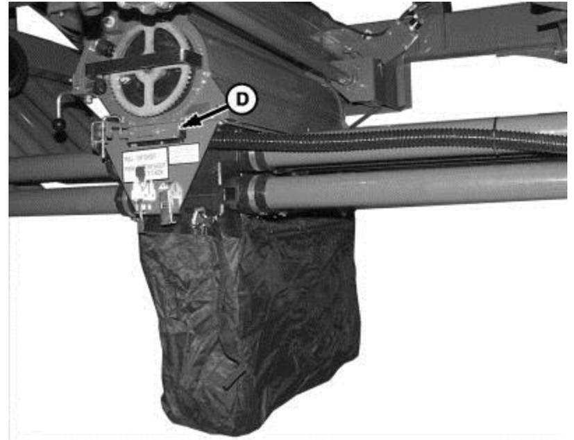
**2. Remove cover plate from bottom of meter and install collection bag.**
