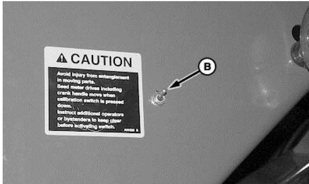
**Activate calibration switch or manually rotate meter handle 12 rotations counterclockwise**
