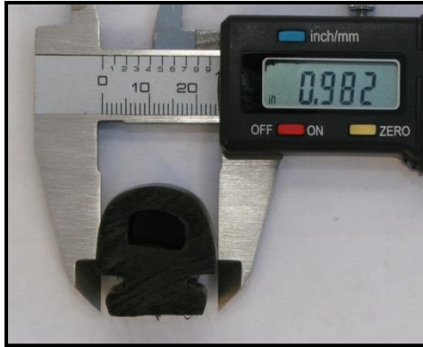
John Deere 1 x 10” Firming Wheel. (fitted on factory drills and seeders from around 1989 to 2006)
