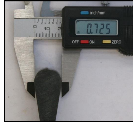
Case IH 0.7 x 9” firming wheel which is optional on a Case SDX 30 or 40 air-seeder.
