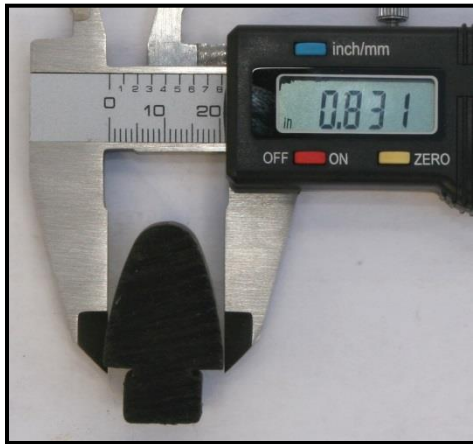
New John Deere 0.8 x 9” Firming Wheel. (fitted on factory drills and seeders from summer 2006).
