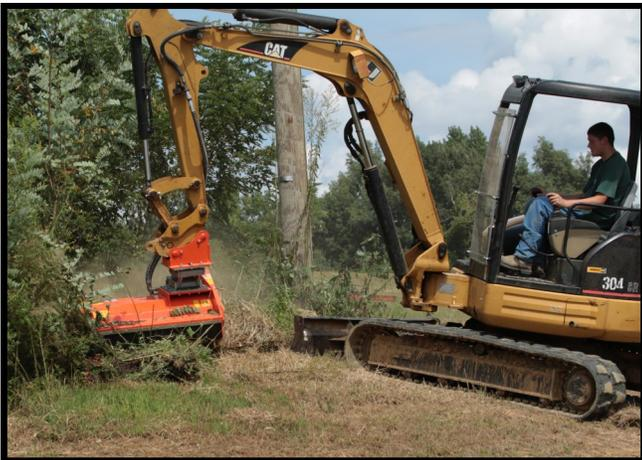
The image to the left shows a Lipa TLBE-100 on a CAT 304CR mini excavator. This 9800 lb machine had a maximum auxiliary flow of 18.5 gallon per minute. The TLBE-100 only requires 15-16 gallons per minute, so we added an optional flow regulating block to regulate the flow down. By adjusting the flow, the rotor speed can be set to around 2300 RPM, to optimize the mower performance and maximize flail life.
